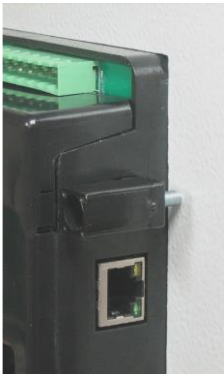
Installation of screw type bracket
